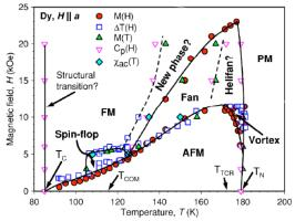
**Fig. 1.** The magnetic phase diagram of single crystal of dysprosium. At least the following phases are present in the temperature range 200 - 80: ferromagnetic, antiferromagnetic, fan, vortex, paramagnetic. Reproduced from A. S. Chernyshov et al. [17], with permission. Copyright (2005), American Physical Society, DOI: 10.1103/PhysRevB.71.184410.
