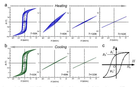
**Fig. 4.** *B-H* hysteresis loops with different amplitudes of the magnetic field *H*, shown at different temperatures during (a) heating, (b) cooling; (c) the hysteresis loop parameters  $B_a^*$ ,  $B_R^*$  and  $W_F^*$  are the maximum flux density, remanent flux density and hysteresis losses, respectively. Reproduced from S. Kobayashi [29], with permission. Copyright (2011), American Physical Society, DOI: 10.1103/PhysRevLett.106.057207.
