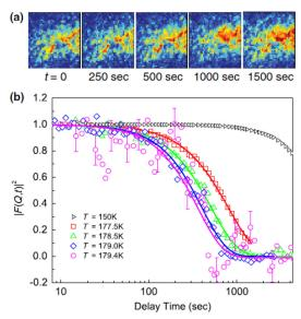
**Fig. 6.** (a) Snapshots of speckles versus time obtained using X-ray photon correlation spectroscopy at 178.5 K for a thin film Y/Dy/Y; (b) normalized autocorrelation function at various temperatures, the rate of change of function as it approaches Neel's temperature becomes higher. Reproduced from S. W. Chen et al. [39], with permission. Copyright (2013), American Physical Society, DOI: 10.1103/PhysRevLett.110.217201.
