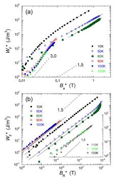
Fig. 5. Relationship between (a) hysteresis losses  $W_F^*$  and maximum magnetic flux density  $B_a^*$ ; (b) between the hysteretic losses  $W_F^*$  and the remanent magnetic flux density  $B_R^*$  at different temperatures during heating, plotted on a double logarithmic scale for a polycrystalline dysprosium sample. Reproduced from S. Kobayashi [29], with permission. Copyright (2011), American Physical Society, DOI: 10.1103/PhysRevLett.106.057207.
